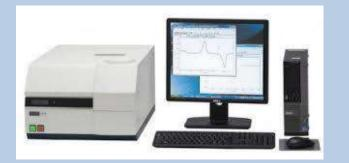
Thermogravimetric Analysis can track the changes in the mass of your sample as the temperature is changed in a controlled manner. Analysis typically consists of monitoring the mass of your sample while heating at a constant rate, or held at a constant temperature over time.
